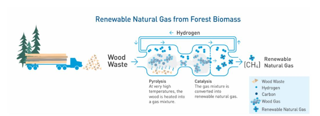
Wood methane made from forest biomass has the potential to supply all of the natural gas consumed in Quebec.
