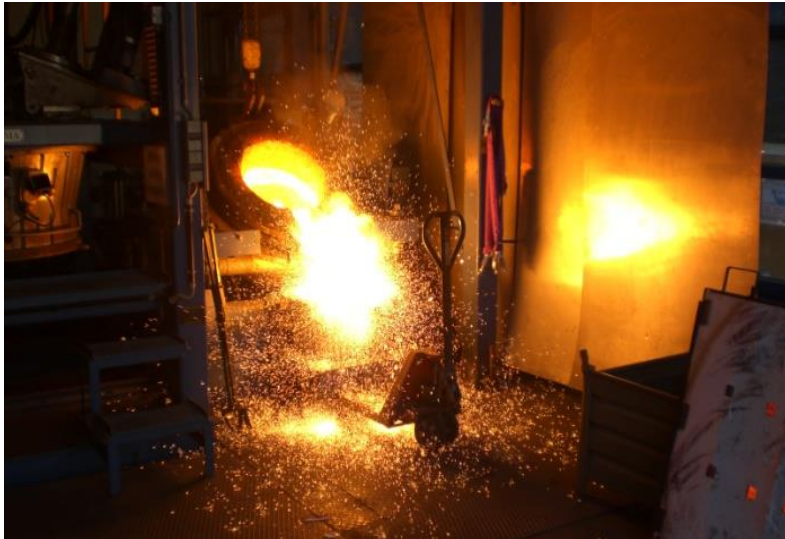
Tapping of a trial melt in the pilot EAF
