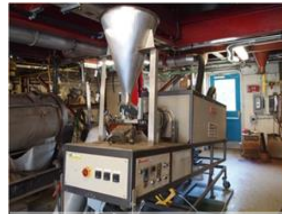
Rotary Kiln Torrefaction, up to 20 kg/h feed rate
