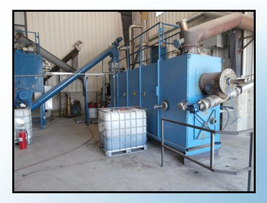
Carbonization of wood chips to fuel separate solid fuel combustors and utilization of residual carbonizer heat via 400 kWt waste heat boiler.
